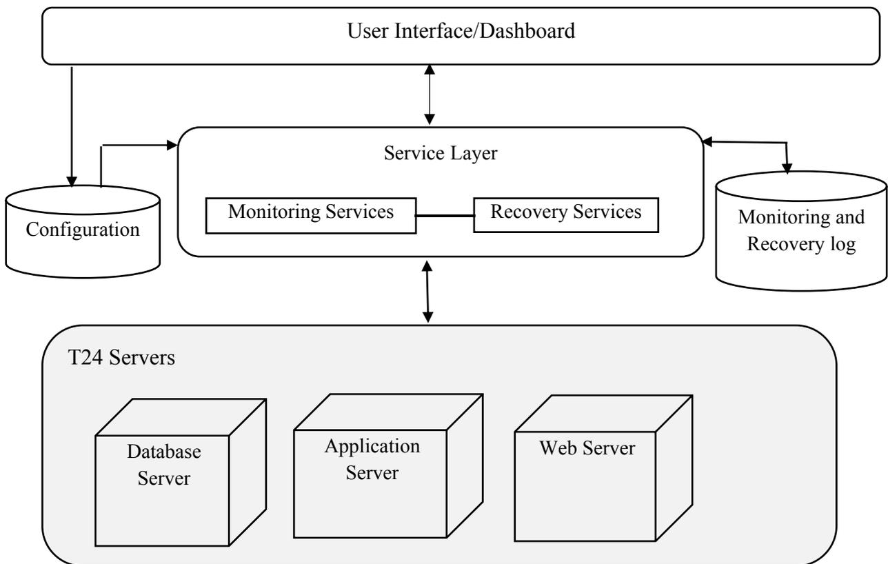
Figure 1: Integrated Monitoring Tool Architecture
