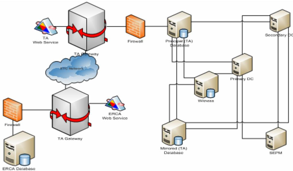
Figure 3: Deployment diagram for DEWS
